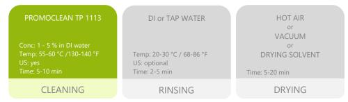
Increasing the bath-life of your process can be achieved by adding an oil separator within the cleaning equipment and to add periodically concentrated product. A PCA Kit is available to monitor the bath status by colorimetric titration.
